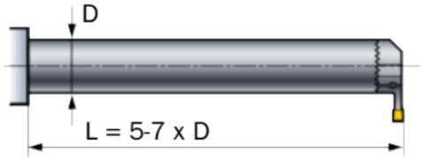
For overhang 3-6 x D use dampened or carbide bars.
