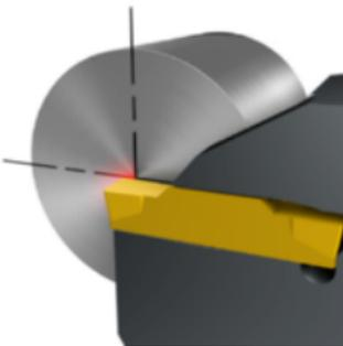
Feeding through centre causes breakage.
