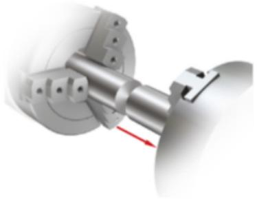
A sub chuck can be used to pull the component.
