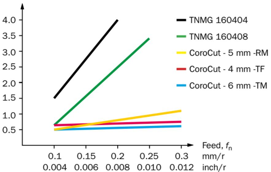
The diagram shows surface finish for CoroCut inserts in comparison to a TNMG insert with a 04 or 08 corner radius.
