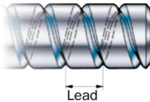
Second threading groove
