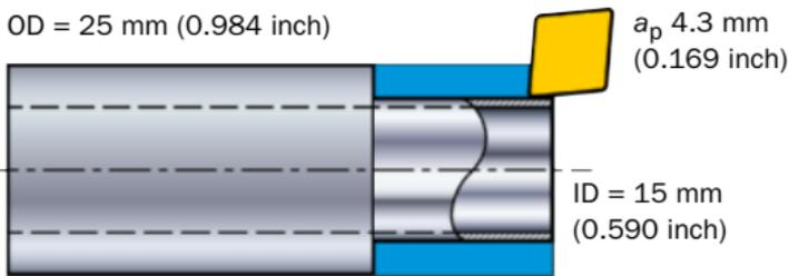
An entering angle close to  $90^\circ$  (lead angle  $0^\circ$ ) can be used for directing the cutting forces in axial direction. This leads to minimal bending force on the component.
