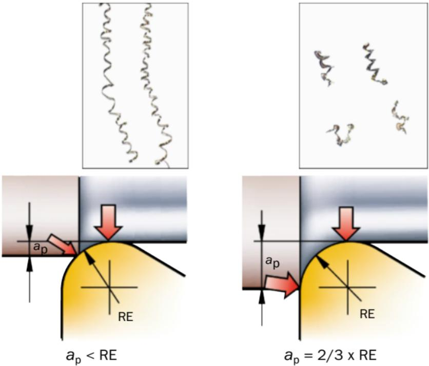
The depth of cut,  $a_p$ , should be no less than  $2/3$  of the nose radius,  $RE$ , to avoid vibration and bad chips.
