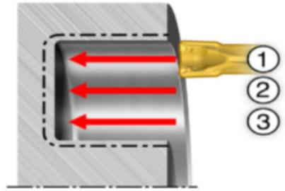
The groove can always be widened by overlapping cuts (or side turning) as long as the first cut is within the diameter range of the tool.
