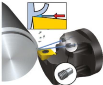
High precision nozzles direct coolant exactly at the cutting zone.
