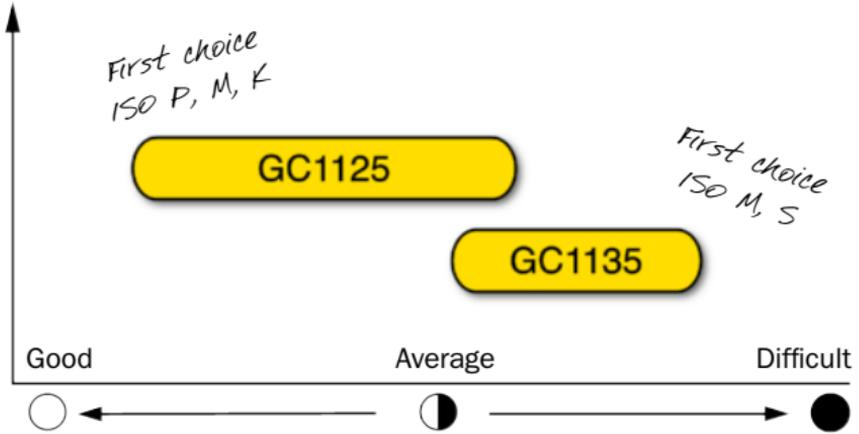
Use GC1125 grade if higher need of heat resistance, because of higher cutting speed and longer engagement time.
