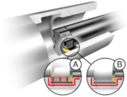
For overhang 5-7 x D use carbide reinforced dampened bars.
