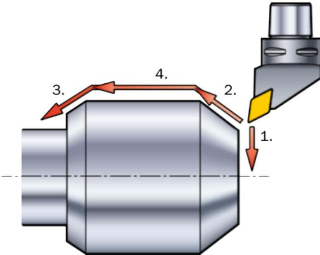
Facing shall be the first operation to set the reference point on the component for next pass.
